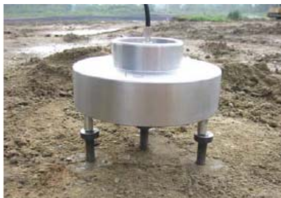
Figure 2.22 Multi-needle heat-pulse method for field tests (Puedue University School of Civil Engineering, 2002)
