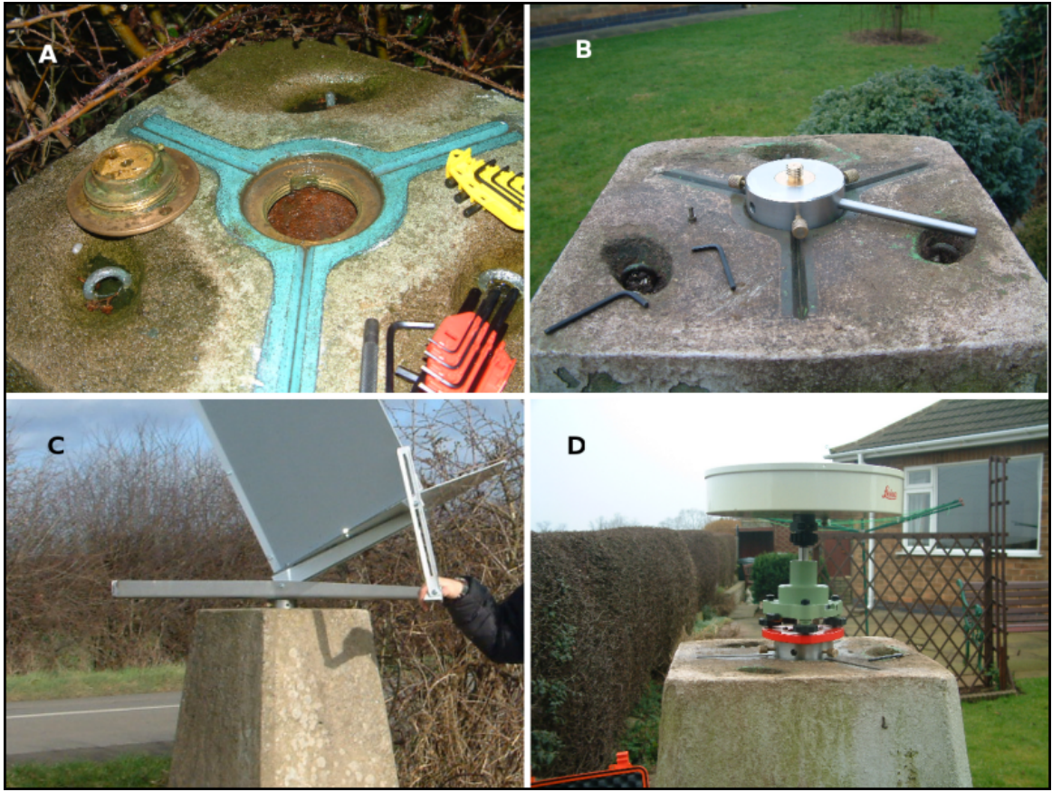
Figure 5.3: The OS pillar mount. (A) An OS pillar with the thread exposed. (B) The mount fitting into an OS pillar. (C) A reflector with modified base in the mount. (D) A GPS antenna in the mount.
