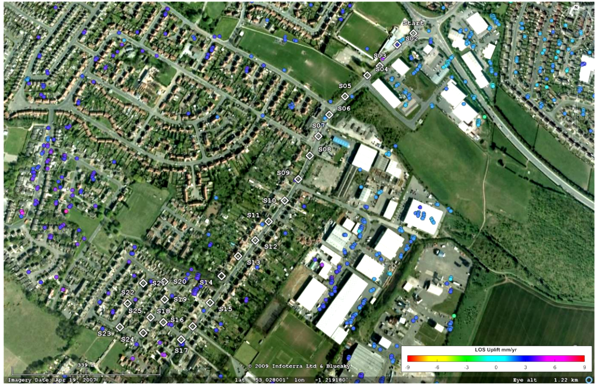
Figure 7.13: The Hucknall precise levelling campaign. White diamonds show the staff positions observed four times of the twelve month period from August 2007 to August 2008, coloured dots represent the PS points.
