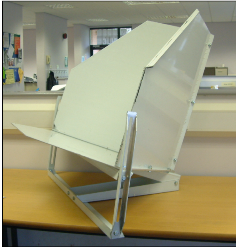
Figure 5.1: Trihedral corner reflector used in the NCRA, supplied by NPA. The reflector has an adjustable elevation and has sides measuring 0.8m from apex to apex making them transportable by car.
