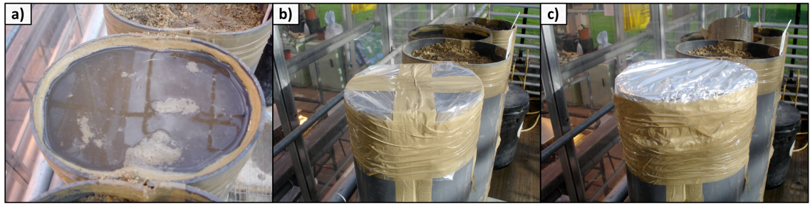
Figure 3.5 Procedures to achieve the field capacity (FC) in soil columns: irrigation to saturation (a) and closure of the top with plastic bag (b) and kitchen foil (c).
