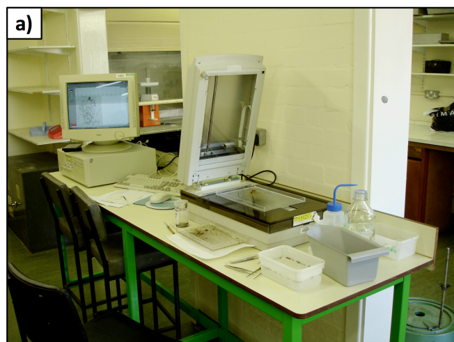
Figure 3.9 Root scanner (WinRHIZO STD 1600+, Regent Instruments Inc., Quebec, Canada) (a) and barley cv. Rum under irrigation and 100 Kg N ha -1 fertilizer root scan (b).
