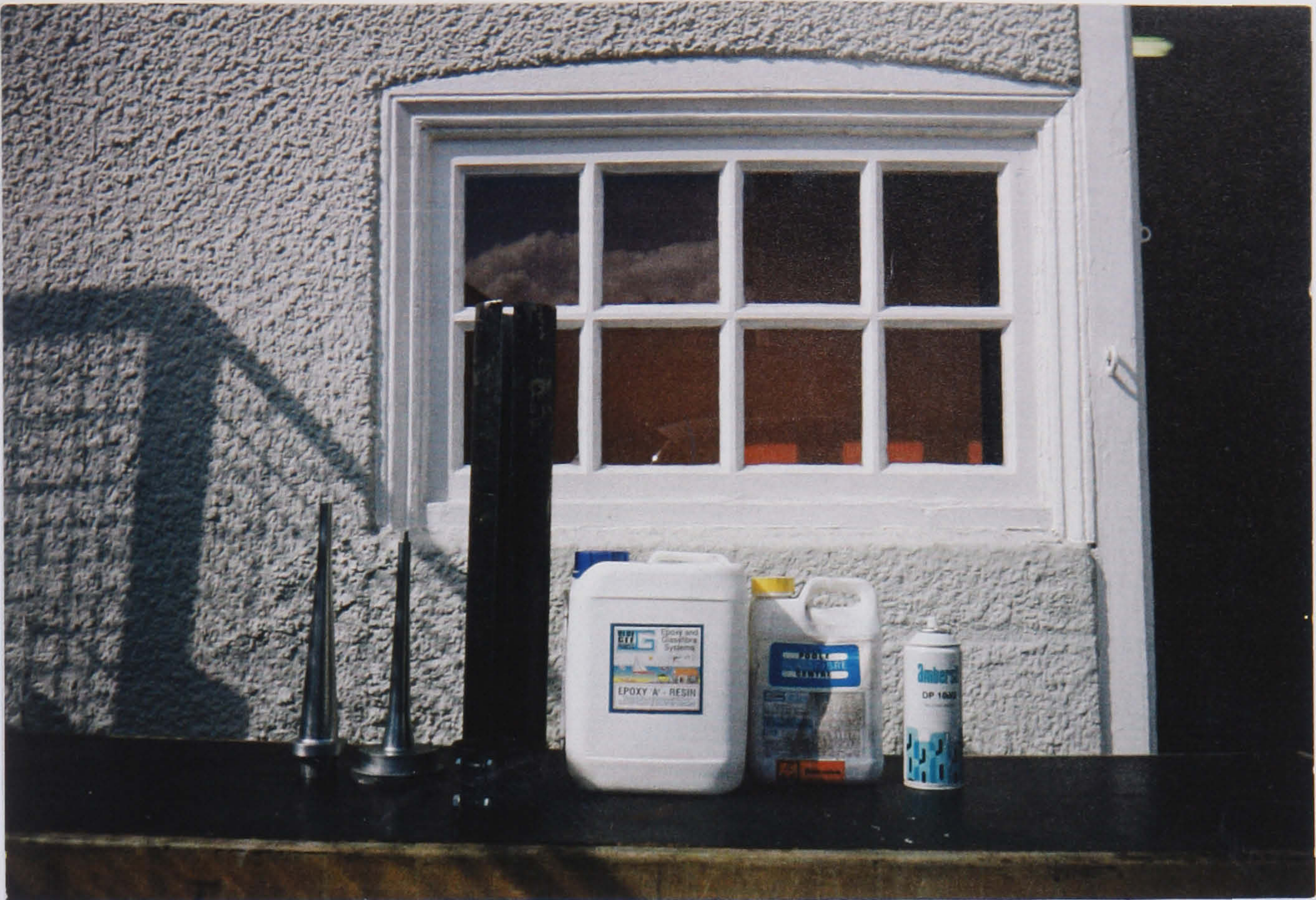
Figure 7.2 (a) Photograph of the two half-formers, sleeve and the epoxy resin system.
