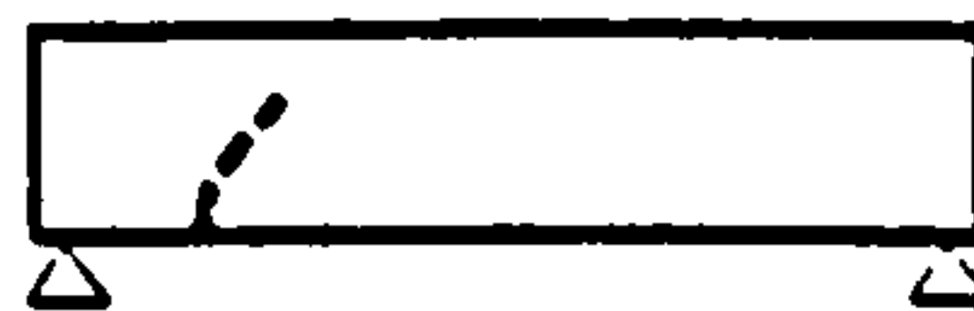
a) Flexural shear cracking of concrete
