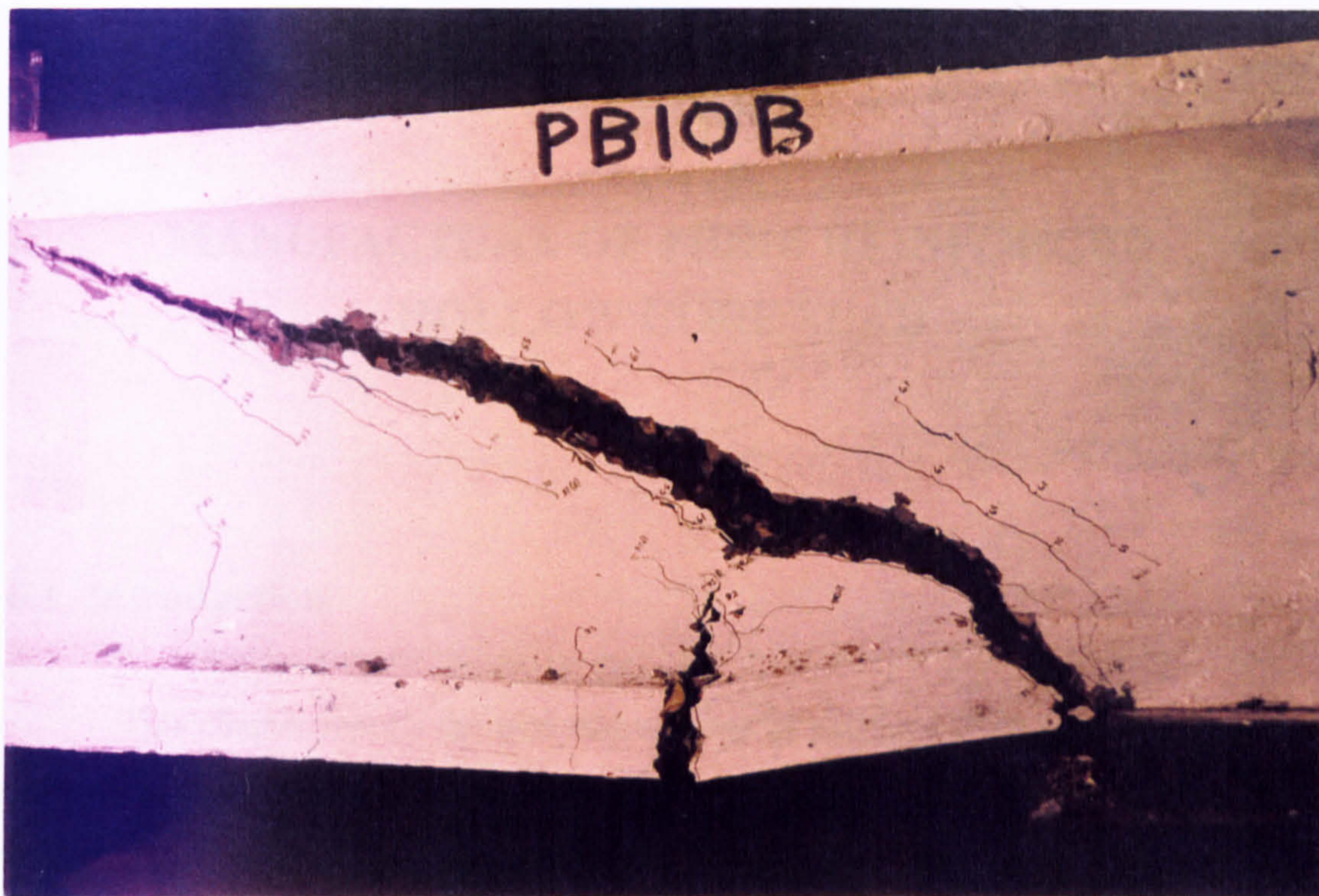
Plate 5-5 “Soffit crack” in beam PB10B
