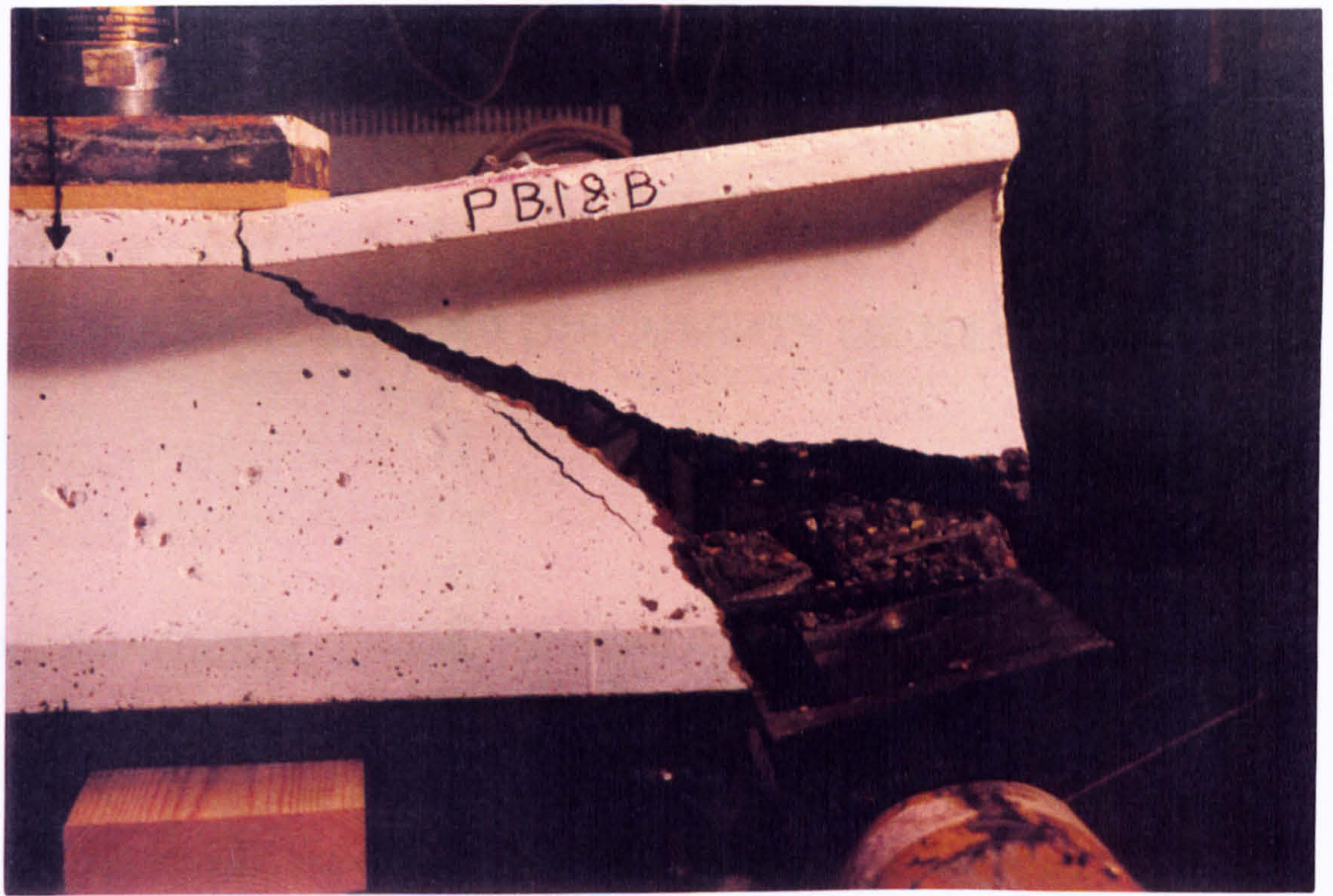
Plate 8-1 Dowel action in plain concrete at large deflections
