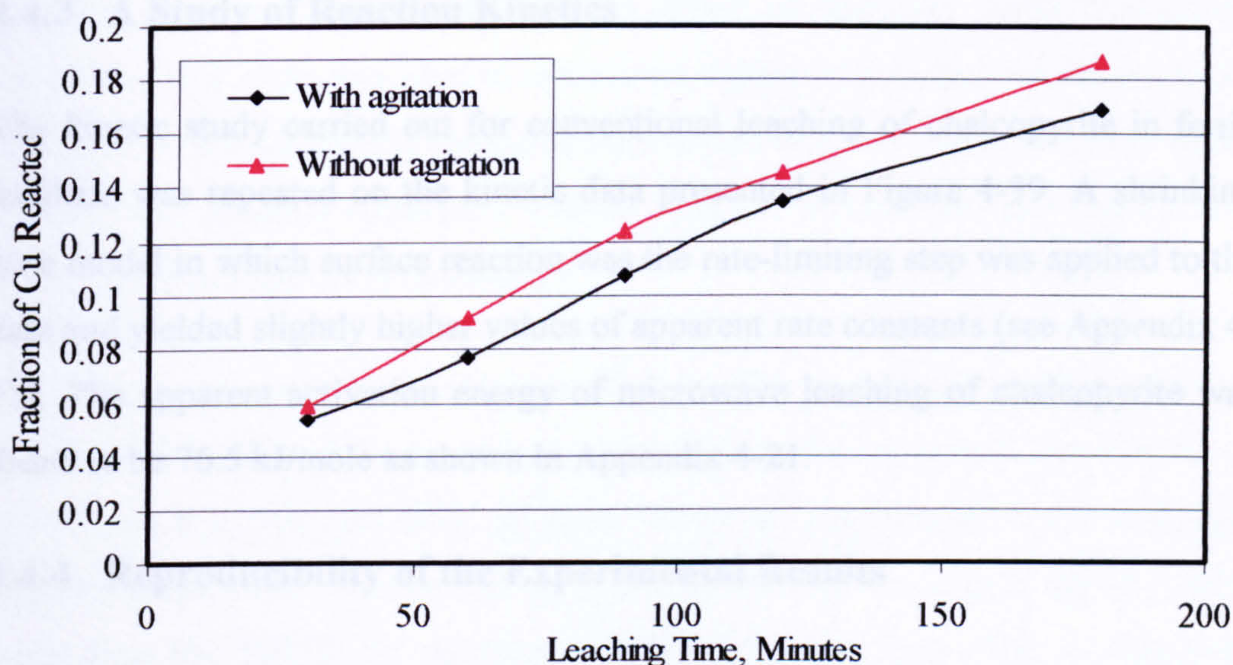
Figure 4-41 Effect of agitation on the amount of copper extracted during microwave leaching of chalcopyrite ( C_{Fe_2(SO_4)_3} : 0.25 M, temperature: 91°C, particle size: <38 \mu m ).
