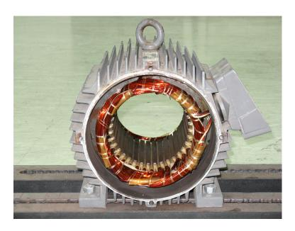
Figure 4.37: Stator of induction machine
