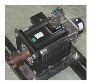
Figure 4.30: Picture of PMSM
