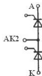
Fig. 5.2: The schematic of the thyristor module used in the prototype
