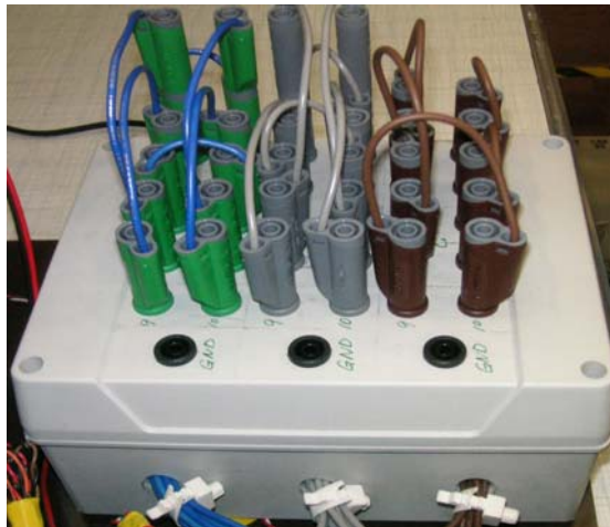
Fig. 5.17: Photograph of the switch box showing the interconnecting nodes and the bridge wires
