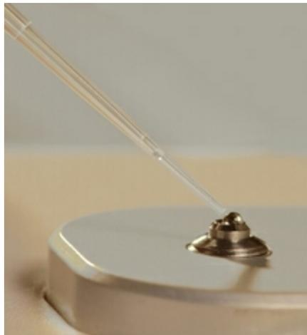
Figure 6 - Nanodrop sample application. With the sampling apparatus open, a droplet of sample is pipetted onto the lower measurement pedestal
