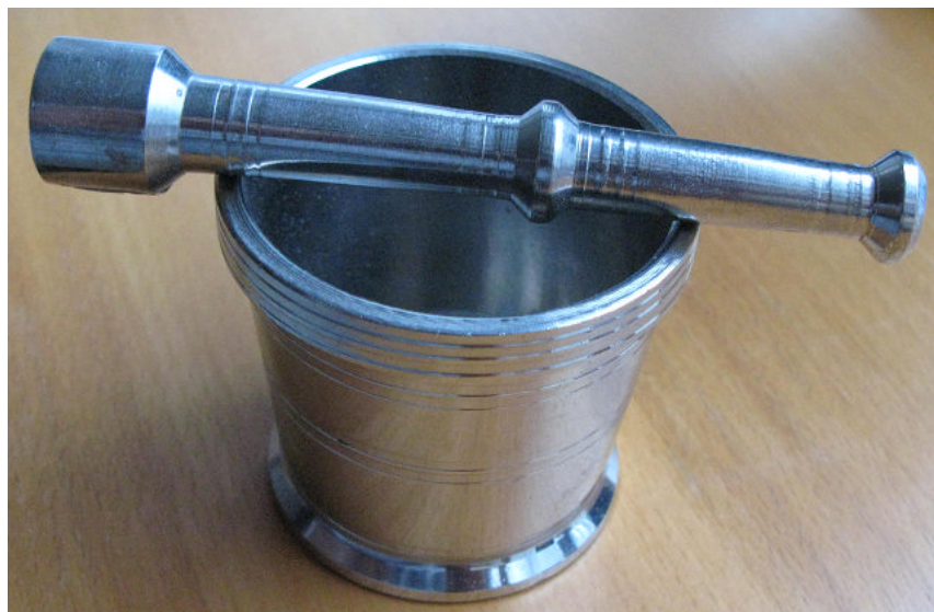
Figure C-6. Steel mortar and pestle used for crushing silica rods.
