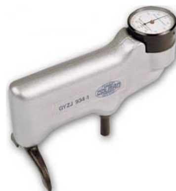
Figure 2-9. Barcol hardness tester.
