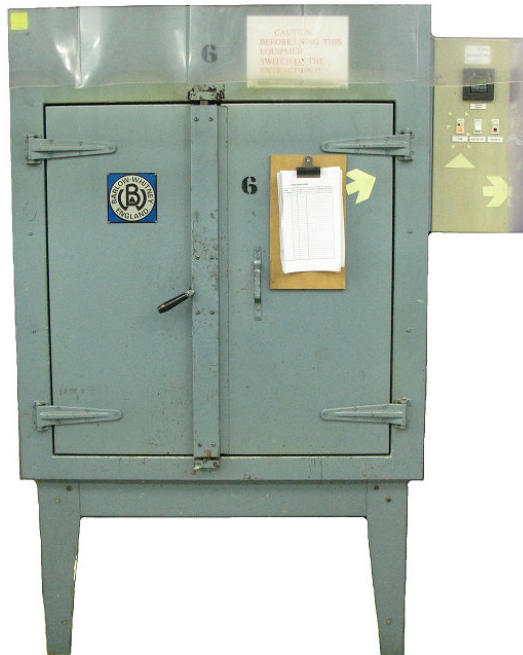
Figure C-5. Barlow Whitney oven used for heat treatment of the fibre samples wound on the aluminum tool (Figure 5-1 of Chapter 5).
