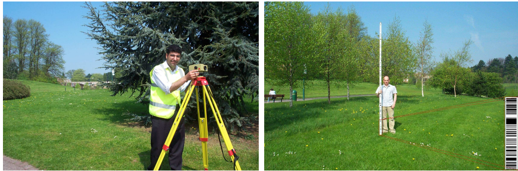
Figure A1.4: The author working with the Wild NA2000 automated digital level (left) and a colleague holding the bar-coded invar level staff (right)
