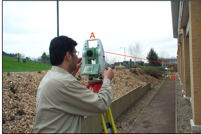
Figure A1.6: The author conducting the Zero Error Test using the Leica TCR1201 total-station
