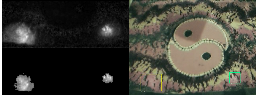
Fig 5.9 – Operator output (top left, scaled for clarity). Candidate regions resulting from use of Rosin's thresholding technique (bottom left, again scaled for clarity) are found to be in line with a user's perception of the extent of flashlight beams.
