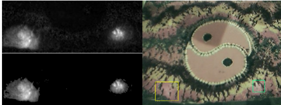
Fig 5.6 – The operator output (top left, scaled for clarity) is extreme sensitive to light making it possible, using the above described technique (bottom left, again scaled for clarity), to determine more of a beam's extent than a human might. This however may not be in line with a user's perception of the extent of a beam (marked right).
