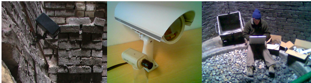
Fig 4.9 – i) Cameras fixed to an original pipeline within custom made housings designed both to protect and camouflage them. ii) The equivalent smallest available commercial solution is too large, heavy and conspicuous to be suitable for use at Etruria. iii) Cold and snowy working conditions within the kiln
