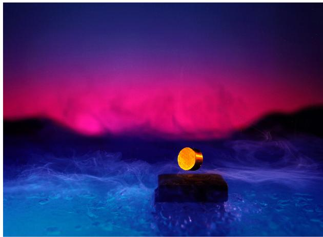
**Figure 2- 22: Photograph showing levitation of a magnet above the superconductor,  $\text{YBa}_2\text{Cu}_3\text{O}_{7-x}$ .**<sup>45</sup>
