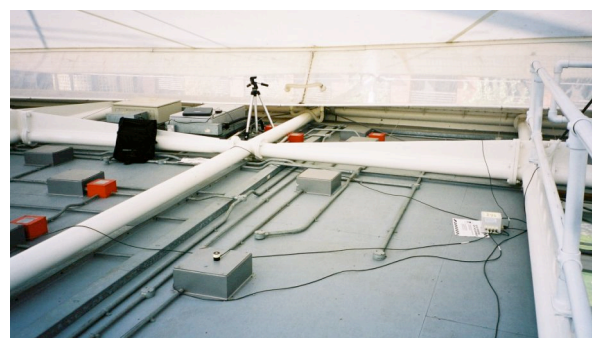
Fig. 4-29 Experimental apparatus on field studies. Above: National Cricket Academy. Upper right: Lord's cricket school. Right: preliminary study in IRAB included readings taken over interior roof at 6m high.
