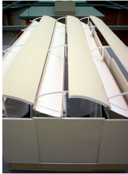
Fig. 5-9 Roof of scale model with three fabric pieces
