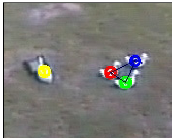
Figure 5.13 Example output frame from the MPS tracker. Three of the four targets’ movements are correlated above the threshold level, and hence three of the targets are grouped together as indicated by the lines – this is an example of automatic grouping as a consequence of the algorithm.
