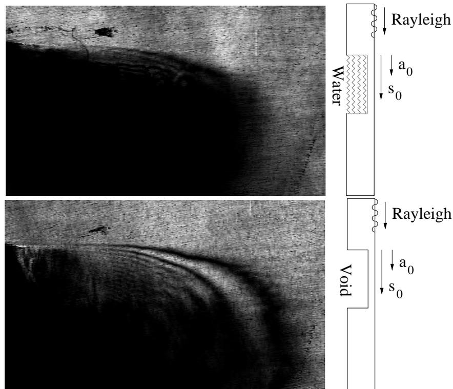
Figure 6.20: The upper 82MHz SAW amplitude image is of a  $1^\circ$  sub-surface slit, with the void behind the slit filled with water. At least one of the Lamb modes is severely dampened in this case by the water. The lower image is of the same region on the sample, but with the water drained out.
