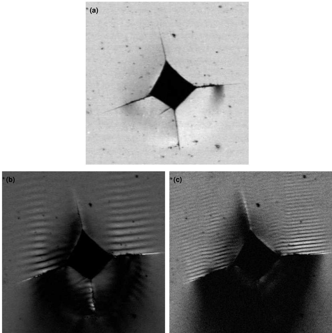
Figure 5.4:  $0.8 \times 0.8$ mm images of a Vickers hardness test indentation on a silicon nitride sample. The three images are as follows: (a) optical image; (b) 82MHz SAW amplitude image; (c) 164MHz SAW amplitude image. The resolution is  $1 \times 1 \mu\text{m}$
