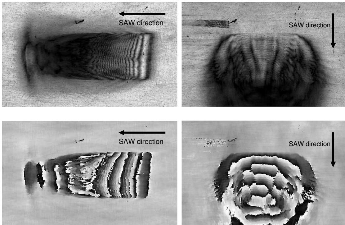
Figure 6.17: SAW 82MHz amplitude (top) and phase (bottom) images of the ‘circular profile slit’ shown in figure 6.15. In the left hand images, the SAWs are travelling from right to left, as indicated by the arrow. In the right hand images, the SAWs are travelling from top to bottom. The left hand images are  $7.5 \times 4.5\text{mm}$ , the right hand images are  $7 \times 4.5\text{mm}$ .
