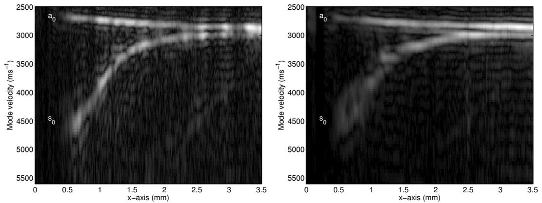
Figure 6.12: Fast Fourier transform (FFT) of the complex amplitude of the SAWs propagating over the  $1^\circ$  slit. The left hand image is from the data acquired by propagating a plane wave, the right hand image is from the data acquired by propagating a focused wave, and is identical to figure 6.6. The  $a_0$  and  $s_0$  modes are labelled.
