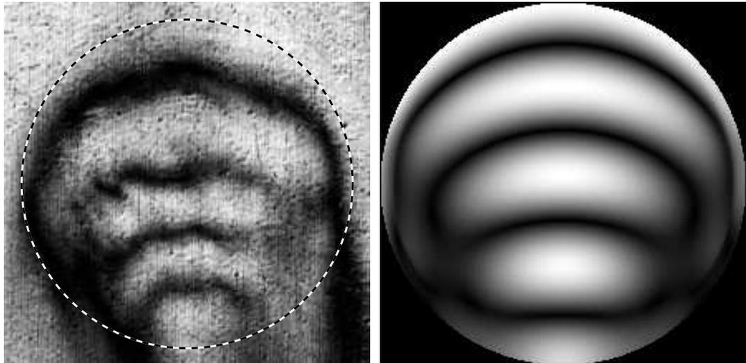
Figure 6.19: The left hand images in an 82MHz SAW amplitude c-scan of a  $1.1 \times 1.1$ mm area of polished aluminium, under which lies a 1mm diameter hole. The approximate location of the hole is marked by the dashed circle. The right hand image is the predicted amplitude response.
