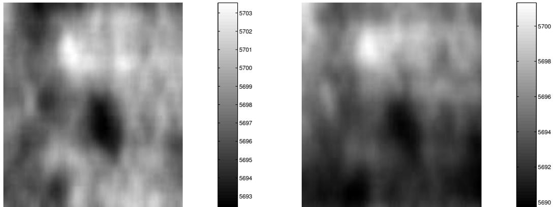
Figure 5.7: 11.5×16mm mean velocity images of a silicon nitride sample. The left hand image is derived from 82MHz SAW phase, the right hand image is derived from 164MHz SAW phase. The source → detector separation is 2mm, and the data has been spatially filtered to approximately this resolution.
