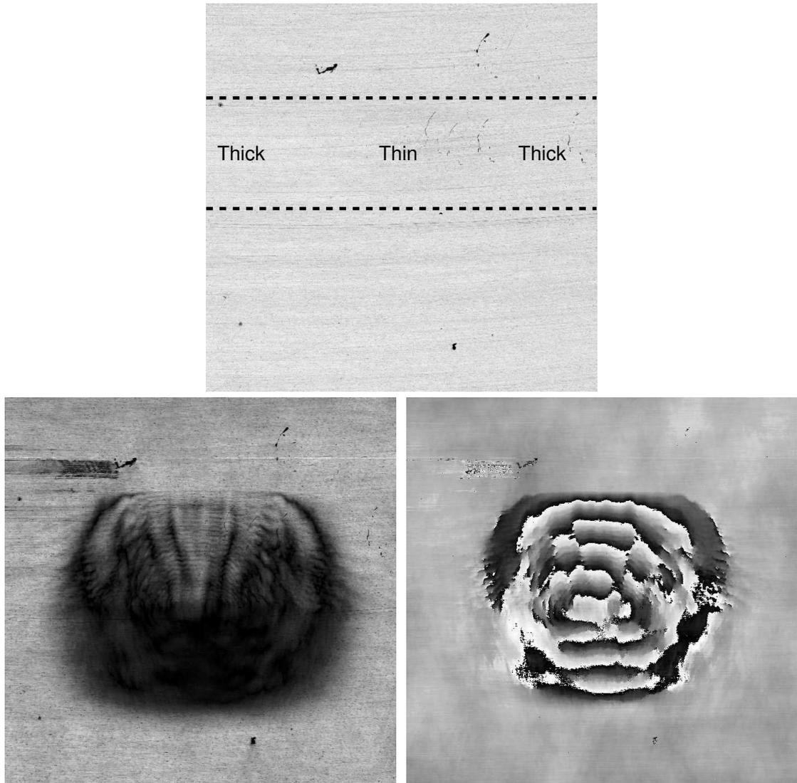
Figure 6.15: Optical (top), 82MHz SAW amplitude (lower left) and 82MHz SAW phase (lower right) images of a  $7 \times 7$ mm area of the top surface of a piece of polished aluminium. The location of the slit is shown by dashed lines in the optical image. The slit is thinnest at the centre (horizontally) of the image.
