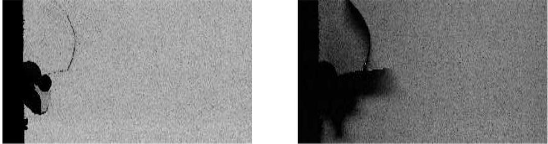
Figure 5.2: Optical (left) and 82MHz SAW amplitude (right) images of a large block of silicon nitride, which contains an optically-visible crack, as well as a finer crack that is invisible at this resolution. Image size is  $20 \times 11.5$ mm, resolution is  $50 \times 100 \mu\text{m}$
