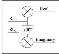
Figure 4.3: Block diagram showing how two mixers may be used in quadrature.
