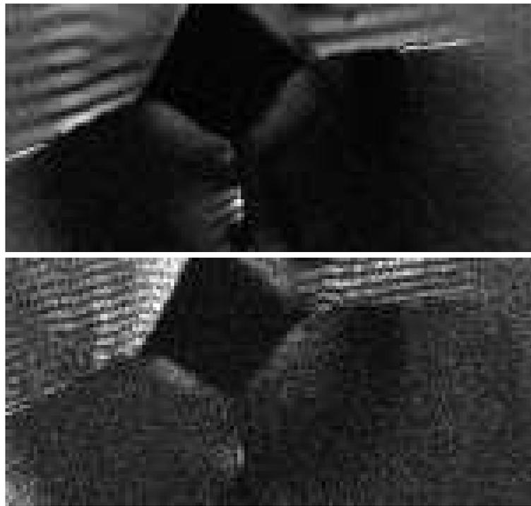
Figure 2.8: Rayleigh wave amplitude c-scans acquired in March 1998 at 82MHz (top) and 164MHz (bottom) of a Vickers hardness test indentation on silicon nitride. The image size is  $750 \times 350\mu\text{m}$ , the pixel size is  $5 \times 5\mu\text{m}$ . The images took around three hours to obtain.
