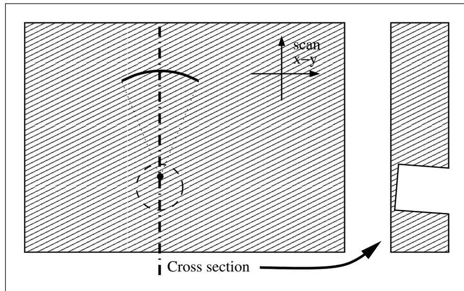
Figure 6.18: Schematic of the ‘hole experiment.’ A 1mm diameter hole is drilled into base of a piece of polished aluminium at an approximate  $1^\circ$  angle. The sample is scanned in the x-y directions to achieve a normal c-scan. The vertical dimension and slit angle in the cross-section diagram have been greatly exaggerated.
