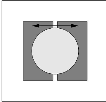
Figure 3.23: A split photodiode, as used in the modified knife edge detection system.
