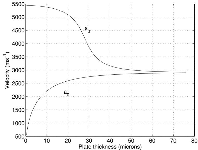
Figure 6.2: Phase velocity dispersion curves for the  $a_0$  and  $s_0$  Lamb modes at a fixed frequency (82MHz) on aluminium.
