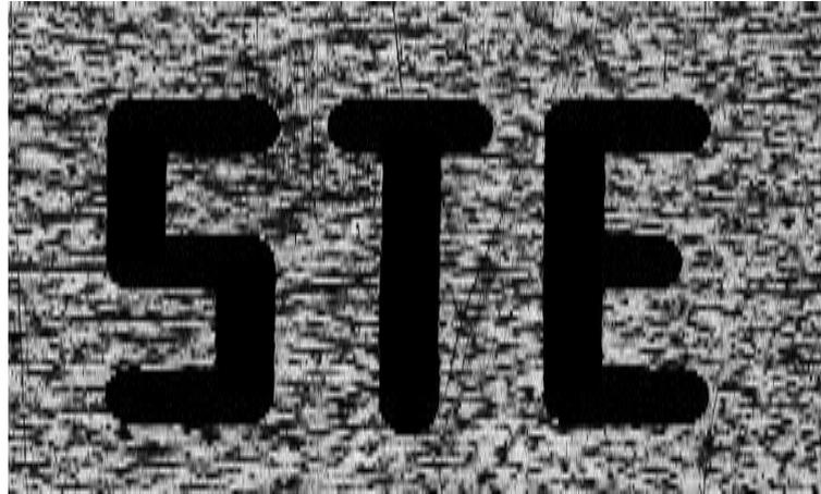
Figure 5.11: Optical image—taken using the O-SAM instrument—of the metal mask, through which 31.6nm of gold was evaporated onto a silicon nitride sample. The size of the image is  $15 \times 9$ mm
