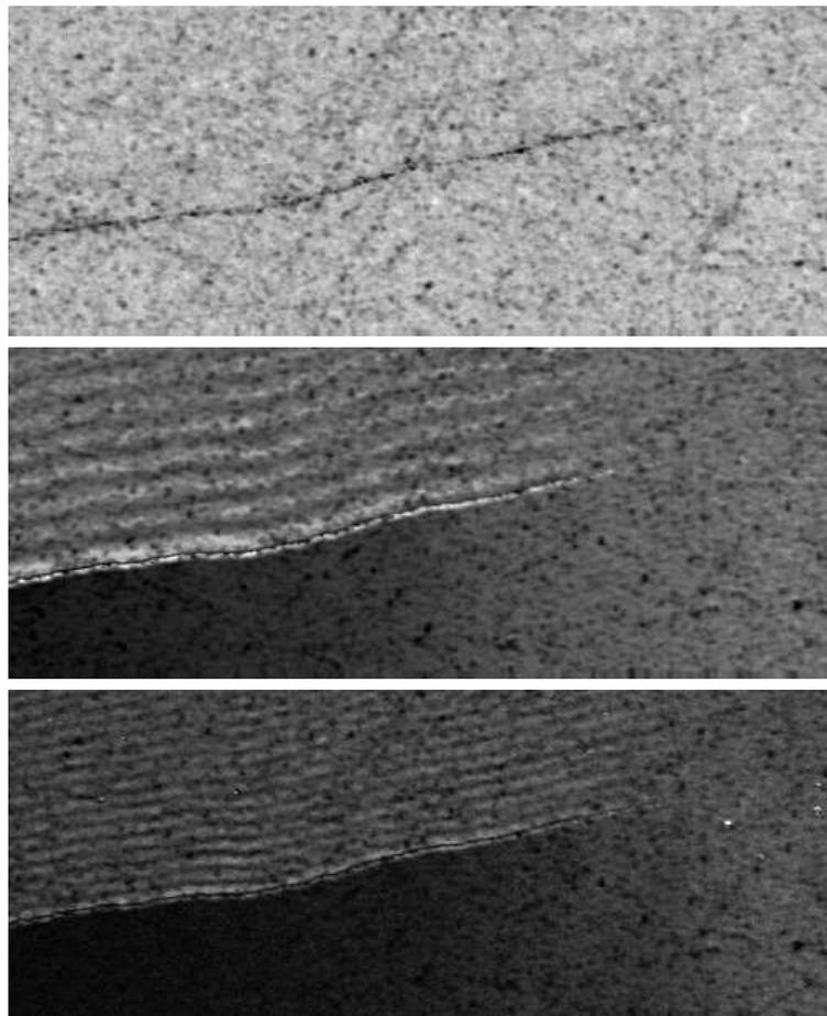
Figure 5.3: Optical (top), 82MHz SAW amplitude (centre) and 164MHz SAW amplitude (bottom) images of a fine crack in a silicon nitride sample. Image size is  $1 \times 0.6$ mm, resolution is  $2 \times 2 \mu\text{m}$
