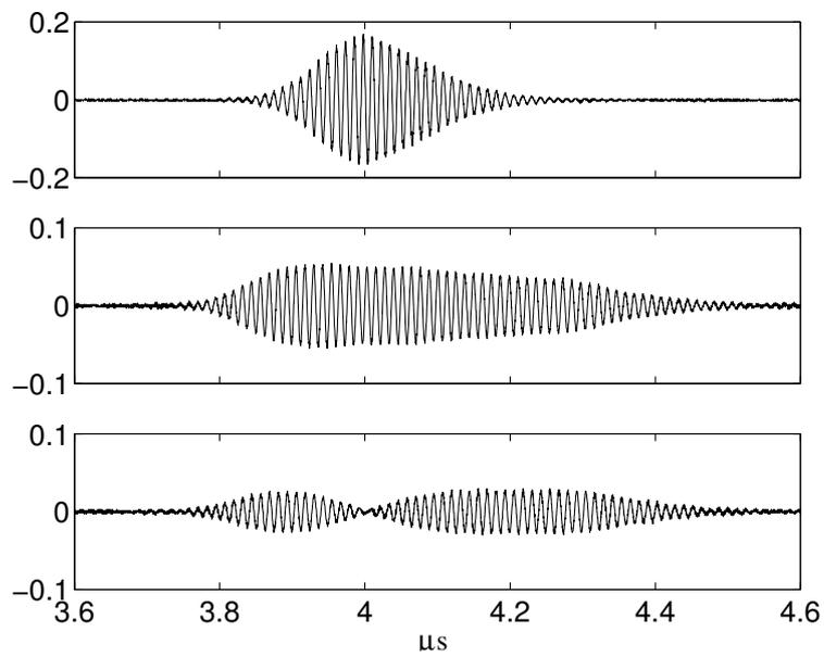
Figure 3.8: The first trace was obtained from the focus of an arc acoustic element and shows no envelope broadening. The second trace was obtained from the focus of the diffractive element shown in figure 3.7. The third trace was obtained from just above the focus of the diffractive element, within a ‘dark lobe.’ The horizontal scale denotes time in  $\mu\text{s}$  since Rayleigh wave excitation.
