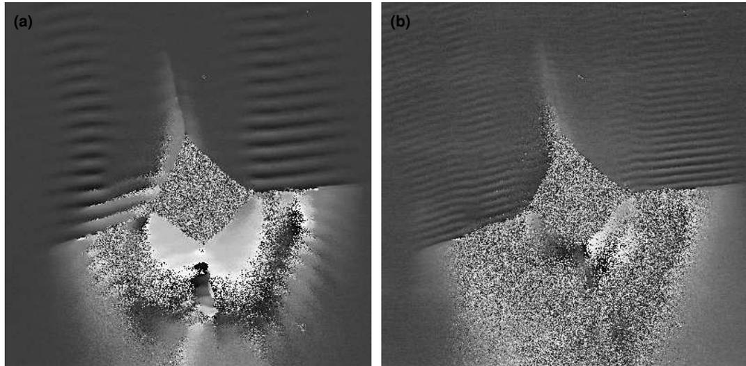
Figure 5.5:  $0.8 \times 0.8$ mm SAW phase images of a Vickers hardness test indentation on a silicon nitride sample, covering the same area as the images in figure 5.4. (a) 82MHz SAW phase image; (b) 164MHz SAW phase image. The resolution is  $1 \times 1 \mu\text{m}$
