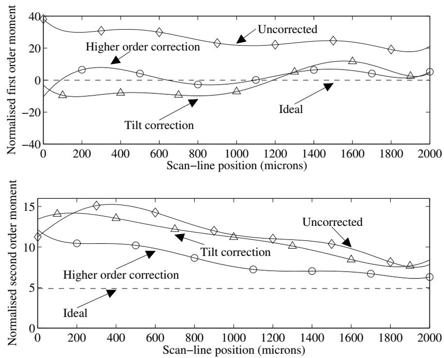
Figure 7.14: The upper plot shows normalised first order moments of the acoustic intensity for uncorrected ( $\diamond$ ), tilt-corrected ( $\triangle$ ) and higher-order-corrected ( $\circ$ ) line-scans. The ideal (- -) is also shown. The lower plot shows the second order moments of the same data. Both plots are best-fit lines through experimental data.
