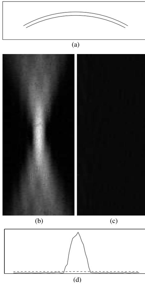
Figure 3.6: Realisation of a surface acoustic wave band stop filter (a), that retains the fundamental frequency of 82MHz inherent in the optical excitation energy and removes the 164MHz harmonic. (b) and (c) show the aerial PSFs at 82MHz and 164MHz respectively. (d) is a line plot through the focus at both frequencies. Aerial PSF size is  $600 \times 300\mu\text{m}$ .
