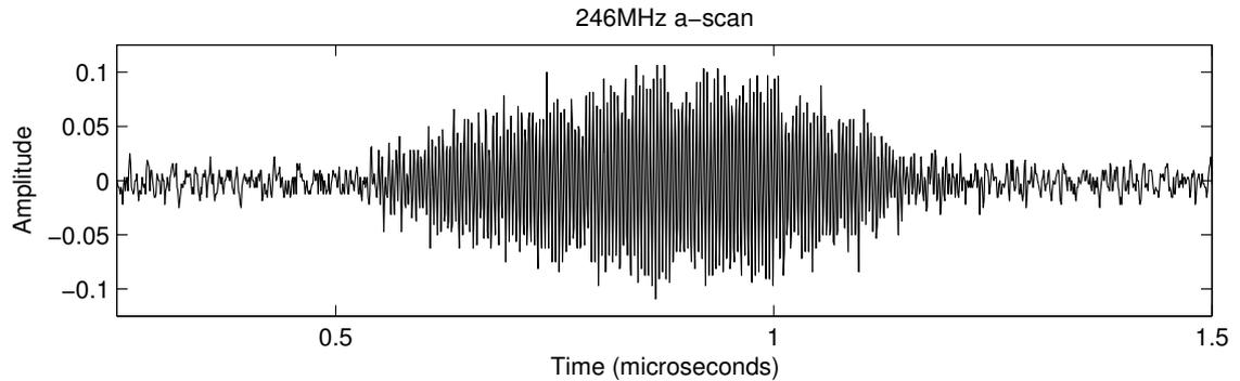
Figure 1.3: An a-scan of a 246MHz Rayleigh wave, acquired with the O-SAM instrument.
