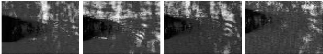
Figure 7.2: Four amplitude images of the same region on an aluminium sample. The only difference between the images is the location of the detection point with respect to the SAW generation region during the c-scans.
