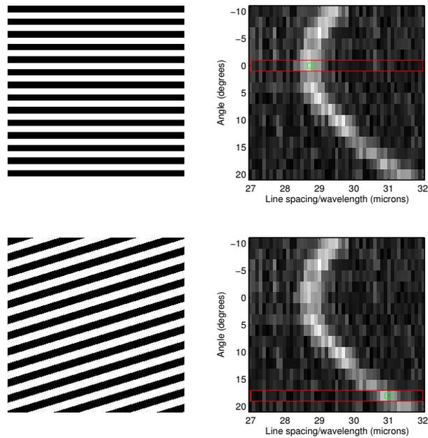
Figure 8.2: Rotating fringe spacing phase velocity measurement technique. Rather than rotating the sample, the image of the fringes is rotated instead.
