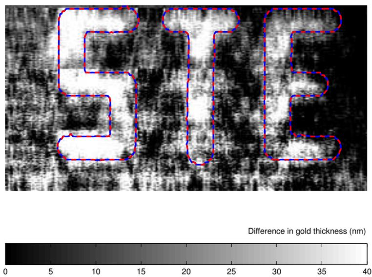
Figure 5.16: Image representing the difference in gold thickness at different points on the area shown. An outline of the mask edges has been artificially added for clarity. The size of the image is  $14 \times 7.2\text{mm}$
