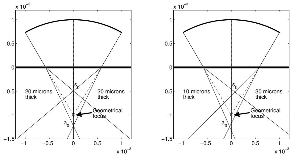
Figure 6.8: The left hand image illustrates the effect of attempting to focus SAWs through a boundary between uniform thick and thin layers. The faster  $s_0$  waves come to a focus before the geometrical focus, whereas the  $a_0$  waves come to a focus after it. The right hand image illustrates the additional effects of propagating through a medium of varying thickness along the x-direction; the foci are now displaced in the x-direction also.
