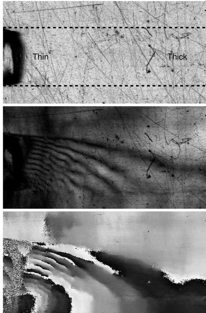
Figure 6.5: Optical (top), 82MHz SAW amplitude (centre) and 82MHz SAW phase (bottom) c-scan images of a  $3.5 \times 1.75$ mm area of the top surface of a piece of polished aluminium. The location of the slit is shown by dashed lines in the optical image. The slit breaks the surface on the left of the image, where the thickness of the aluminium is at its thinnest.
