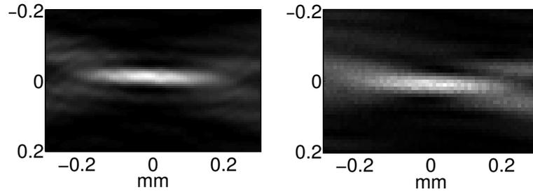
Figure 3.9: Predicted (left) and 82MHz filtered measured (right) PSFs at focus
