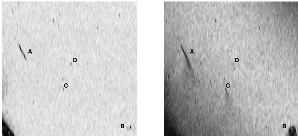
Figure 5.1: Optical (left) and 82MHz SAW amplitude (right) images of a block of silicon nitride, which contains a scratch, and small and large Vickers hardness test indentations. Image size is  $10.5 \times 10.4$ mm, resolution is  $20 \times 200 \mu\text{m}$
