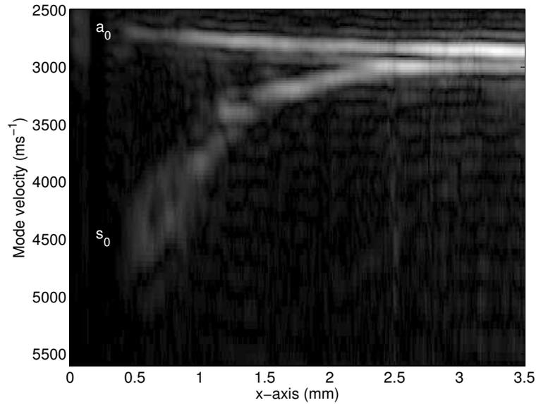
Figure 6.6: Fast Fourier transform (FFT) of the complex amplitude of the SAWs propagating over the slit shown in figure 6.5. The result has been transformed to show velocity rather than spatial frequency. The  $a_0$  and  $s_0$  modes are labelled.
