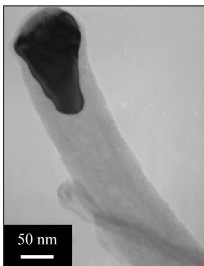
**Figure 2-6 TEM showing the appearance of a CNF grown from the interaction of iron with ethylene-hydrogen (1:4) at 600 °C (Krishnankutty *et al.*, 1996)**
