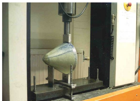
Figure 3.14 Jet engine nose cone mechanical test apparatus.
