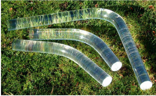
Fig. 4 - 24: Rods with varying bend severity
