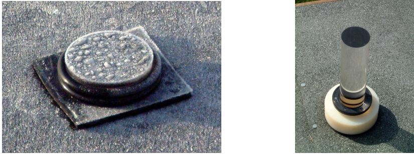
Fig. 4 - 9: Gasket with ring and nylon mount unit on the chamber roof
