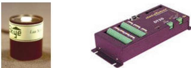
Fig. 3 - 20: Skye SKL310 lux sensor and Datataker DT500
