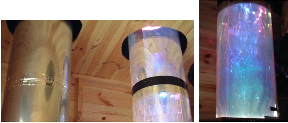
Fig. 7 - 11: Reference (95%) and 98% reflectance light pipes
