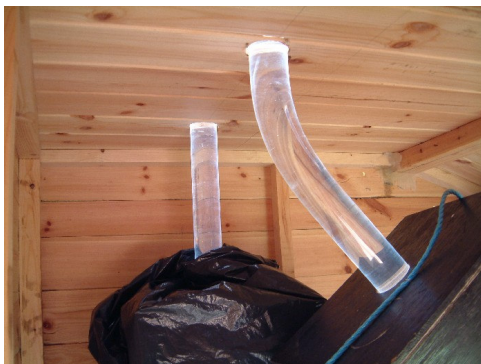
Fig. 4 - 20: Curved rod monitoring in daylighting chamber
