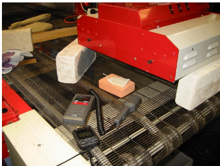
Fig. 4 - 18: Heater and IR thermometer
